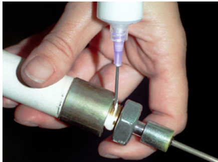
Ceramabond™ 671 used as a high temp threadlocker.
